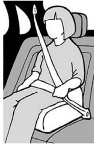
Correct belt fit with a booster
